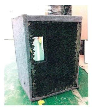
Figure 1: Acoustic Enclosure for Dill, Hand-held (Battery), Circular Steel Saw (Battery) & Grinder, Hand-Held (Battery)
